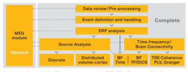
Complete: More tools for: Time-frequency analysis, TSE, ITPL; Coherence, PLV, Granger causality, PDC, DTF; Beamformer (BF), DICS
